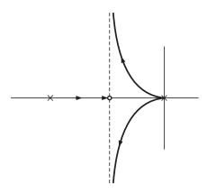
Three roots with nearly equal parts exist on the left half of s-plane.
